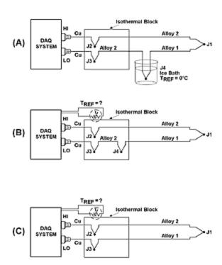
In Figure 2B, we move the reference junction (J4) onto the isothermal block, with the result that the instrument terminals and the reference junction are now at the same temperature. This temperature can be read with a sensor that does not require a reference junction, such as a thermistor or semiconductor temperature sensor.
